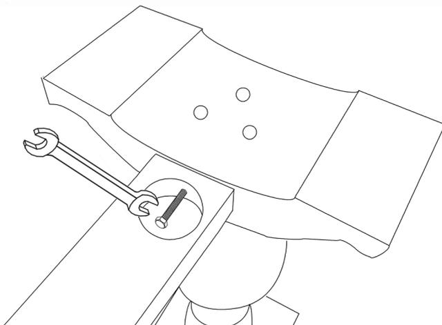
4. After securing the rail to both pedestals, place carefully the table top on a clean, level surface. Afterwards place the pedestals joined by the rail on top of the table top, aligned to the pre drilled holes. Using the 8 bolts, secure the base to the table top.
