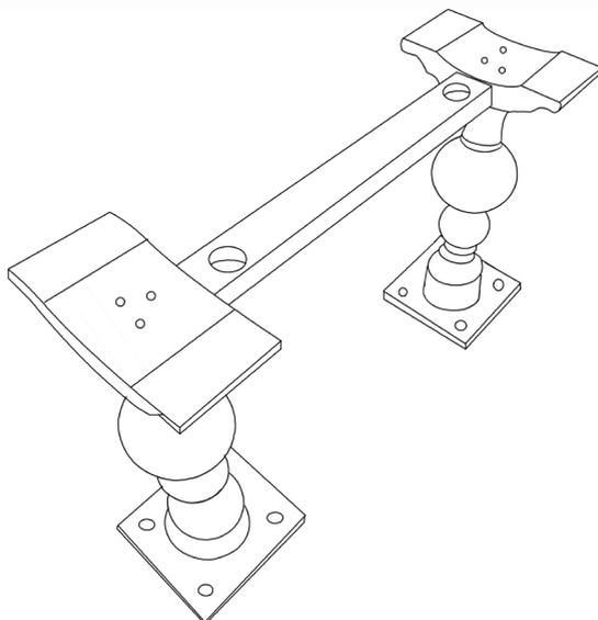
3. Using the tool provided, secure the rail to the pedestals by using the long bolts.
